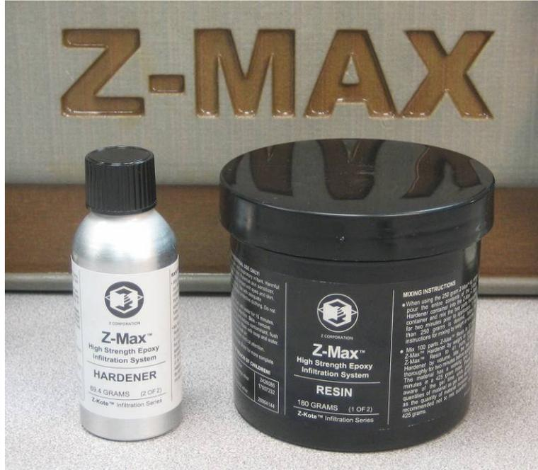
All epoxy infiltration systems benefit from the use of an oven to dry the printed part prior to infiltration. Driving off the excess moisture makes the part more porous, allowing for easier penetration of the epoxy into the part. Z-Max infiltrant penetration depths of 0.25" are possible with a fully dried part.
